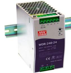
C-WDR240 is a 240W AC/DC compact industrial DIN rail power supply, that features a wide input range for both single and two phase power systems. With a 180 to 550VAC wide input range, C-WDR-240 can be used in general power system with single phase 230VAC input or can capture any two phases from a 330~550VAC three-phase power system.
