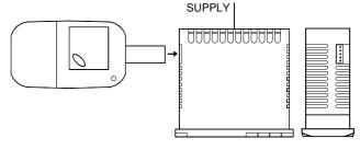
Instrument supplied from the device
